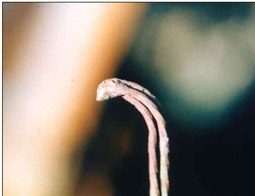
Figure 2 - Arc Faulting of Conductor Harness Continuation Run
