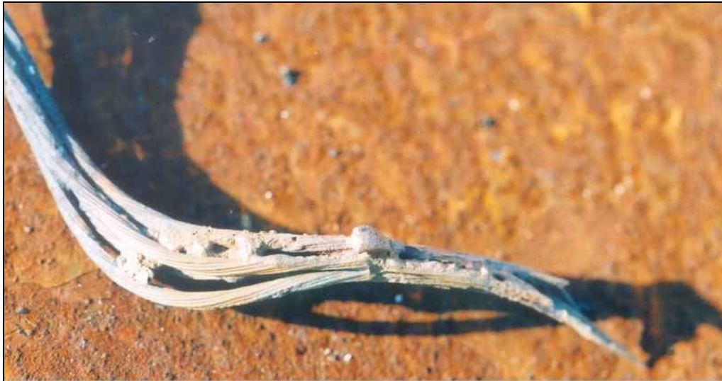
Figure 1 - Arc Faulting of Conductor Harness
