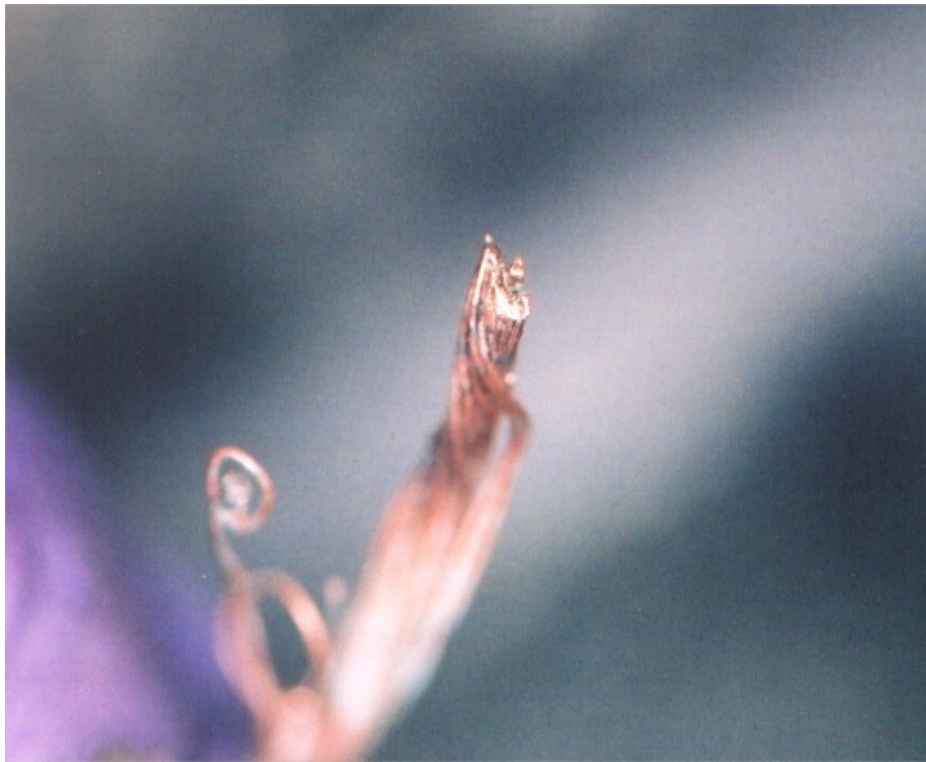
Figure 1 - Melted End of Engine Compartment Harness Conductor
