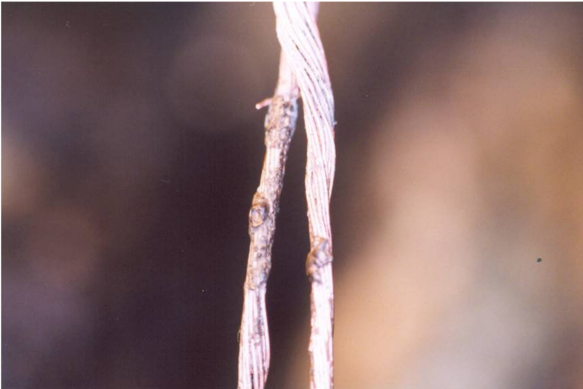
Figure 4 - THROTTLE POSITION SENSOR STRANDED CONDUCTOR FAULTS
