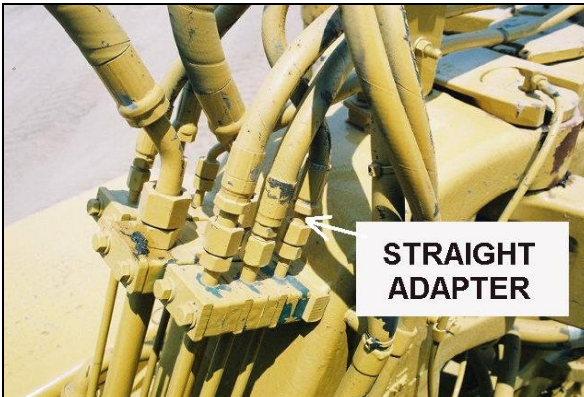
Figure 2 - Straight Adapter (Exemplar - Shown) Versus 45 Degree Adapter (Affected Unit)
